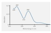
235 and 313nm which are directly proportional to concentration, enabling a series of standards to be produced giving certified absorbance levels between 0.1 and 3.0A. Filter UV20 gives values from **0.1 to 0.3A**, UV40
