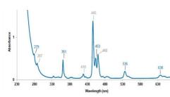
UV and visible wavelength ranges. Standard certification of the F1 Holmium Oxide filter includes the peaks at 279, 361, 453, 536 and 638nm, with optional peaks at 287, 418, 445 and 460nm. The holmium filter is
