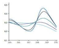
primarily dependent on the slit-width and grating quality. For resolving complex or adjacent peaks having the correct SBW will be vital, and where an application defines a required SBW your spectrometer's performance should be validated using our Toluene in Hexane (UV6) and Hexane Blank (UV9) filters.
